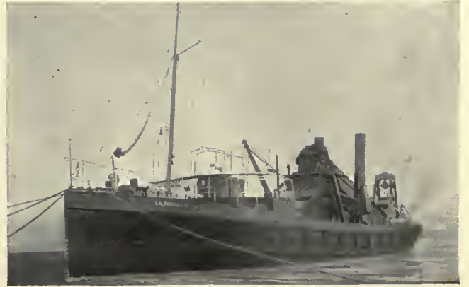
FIG. 4.—Stern-well hopper-dredger "La Puissante," by Wm. Simons & Co. Length 275 ft., breadth 47 ft., depth 19 ft.
